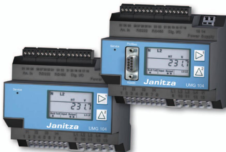
The UMG 104 equipped with a 500 MHz DSP (digital signal processor) is a very fast and powerful power analyser. The continuous scanning of the 8 channels with 20 kHz per channel allows the recording of all electrical parameters (more than 800 values), minimum - and maximum - values, and the main power quality values such as harmonics (up to the 40th, each phase with the detection of direction).
