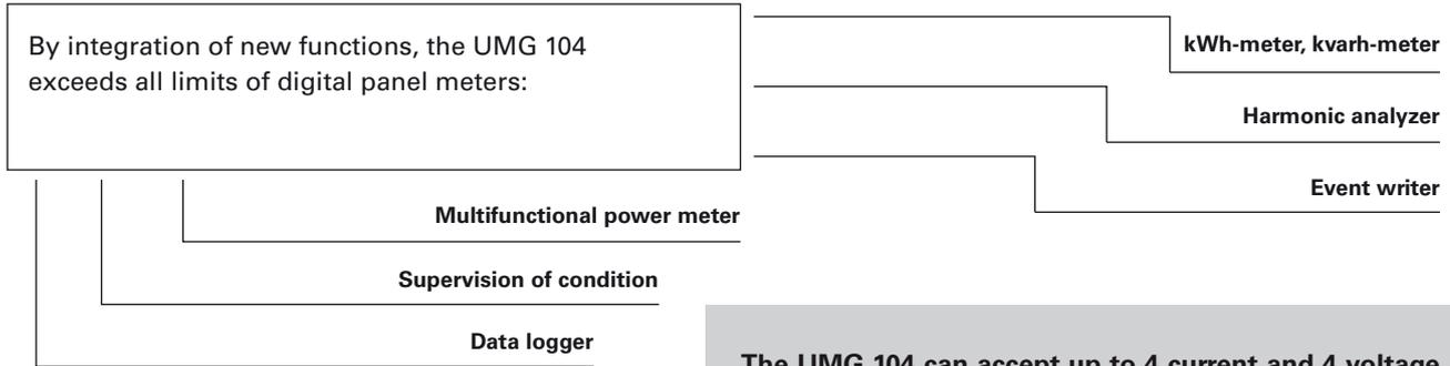
The UMG 104 can accept up to 4 current and 4 voltage inputs, which allows monitoring of up to 4 single phase circuits. Potential applications include data centers, office buildings, motor control centers, etc.
